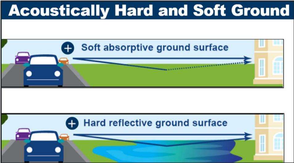
Figure 3 – Characteristics of Ground Surface on Sound
